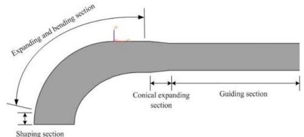
Fig.2 Three dimensional modeling of horn mandrel
