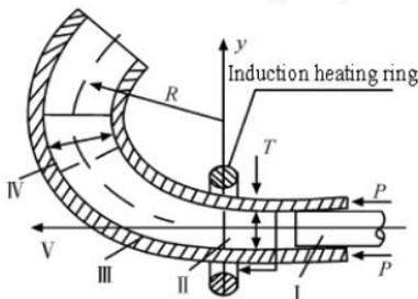
Schematic diagram of hot pushing pipe bending process
